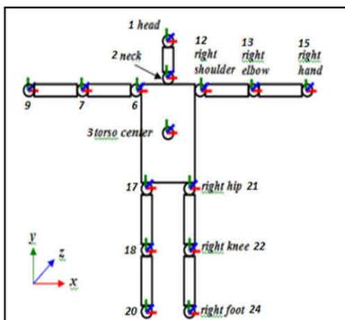
Fig. 2. 24 joint points that Kinect detect 1
